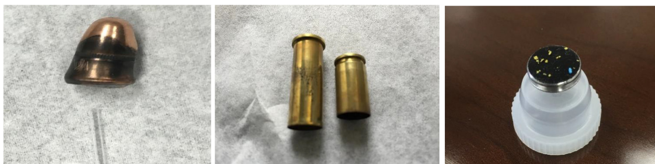
Fig. 2. Categories of trace evidence analyzed in this study. Bullet fired from a gun with a black ABS barrel showing a polymer smear mark and scrape marks from the melting point tube used for DART-MS analysis (left). Cartridge case from the same gun (middle, left shell) showing external black polymer residue, unlike a cartridge case from a traditional gun (middle, right shell). Adhesive stub used to collect GSR and occasionally polymer (colored) fragments from a cotton t-shirt (right).
