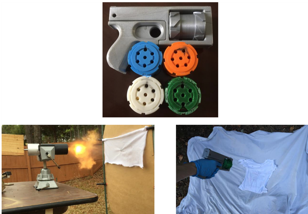
Fig. 1. Phase I test-fire of ABS polymer barrel (left). Fully 3D-printed gun and interchangeable cylinders composed of blue CPE, white ABS, orange PLA, and green PETG (center). Phase II test-fire of 3D-printed gun (right).
