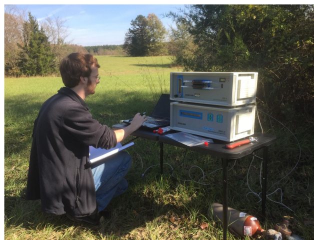
Fig. 2 Field analysis of quadcopter-deployed gold-coated Hg traps by CVAFS
